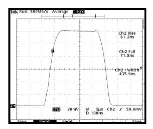
Figure 3-2. Example Of Acceptable Reply Pulse
